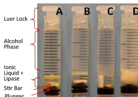
**Fig. 1.** Reaction cells filled with isoamyl alcohol, acetic acid free lipase and bmimPF6 (A) fresh, (B) after thermal treatment, (C) after incubation at 100 MPa, (D) after incubation at 400 MPa.
