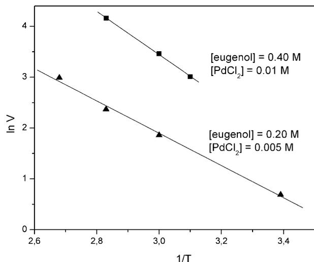
**Figure 1.** Palladium-catalyzed oxidation of eugenol: temperature effect. *Conditions:* gas phase O<sub>2</sub>, 10 atm; solvent DMA/H<sub>2</sub>O (20 vol%).
