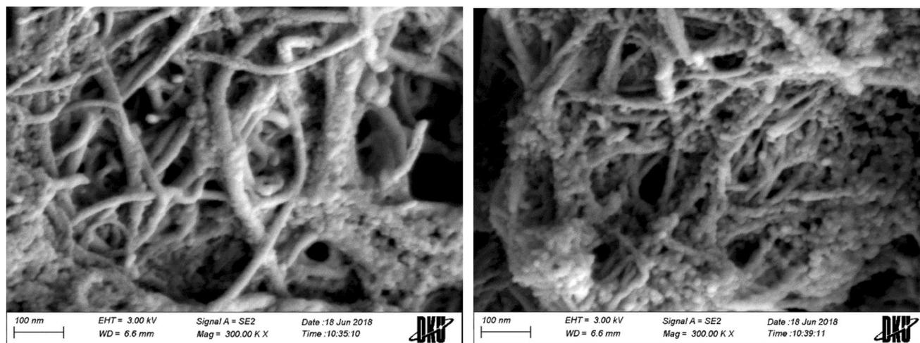
Fig. 2 SEM images of Pd-Chit-CNT; before (left) and after use (right)
