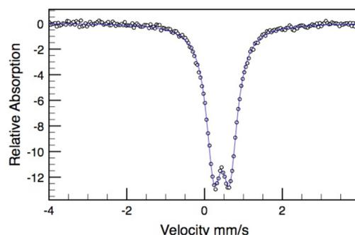
**Figure 3.** 80 K Mössbauer spectrum of BIAN-Fe(C<sub>7</sub>H<sub>8</sub>).
