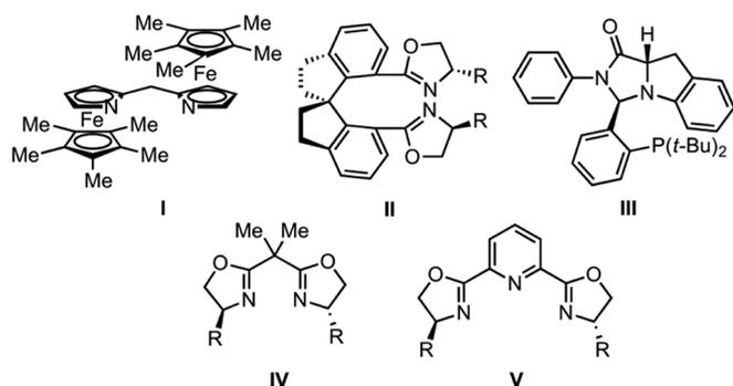
Fig. 2. Reported Bidentate Ligands Used in Cu-Catalyzed O–H Insertions
