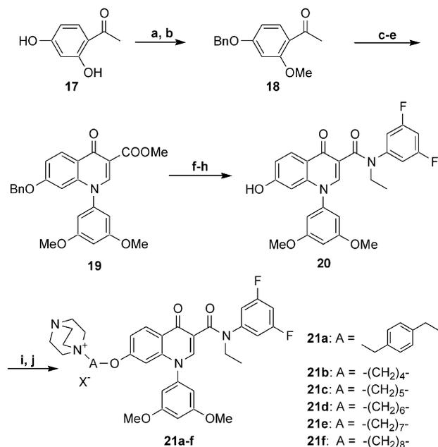
**Scheme 3.** (a)  $K_2CO_3$ , BnBr, acetone (90%); (b)  $K_2CO_3$ , MeI, DMF (98%); (c) NaH,  $CO(OMe)_2$  (86%); (d)  $Me_2NCH(OMe)_2$ ; (e) 3,5-dimethoxyaniline,  $K_2CO_3$ , DMF (73% for two steps); (f) aq NaOH, EtOH (quant); (g)  $(COCl)_2$ , *N*-ethyl 3,5-difluoroaniline (97%); (h)  $H_2$ /Pd-C, EtOH (quant); (i) alkylene dihalide,  $K_2CO_3$ , DMF (67–97%); (j) DABCO, MeCN (53–81%).
