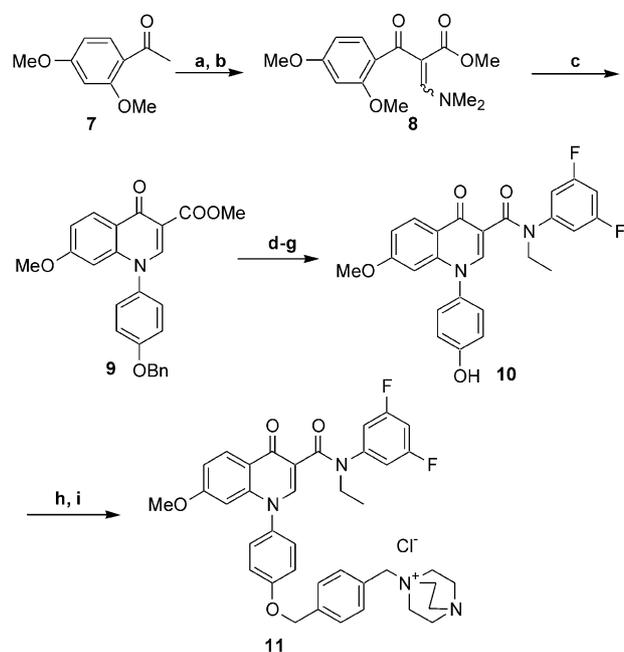
**Scheme 1.** (a) NaH,  $CO(OMe)_2$  (79%); (b)  $Me_2NCH(OMe)_2$  (68%); (c) 4-benzoyloxylaniline,  $K_2CO_3$ , DMF (27%); (d) aq NaOH, EtOH (94%); (e)  $ClCOO*i*-Bu$ ,  $Et_3N$ , 3,5-difluoroaniline (quant); (f) NaH, EtI, DMF (83%); (g)  $H_2/Pd-C$ , EtOH (95%); (h)  $\alpha,\alpha'$ -dichloro-*p*-xylene,  $K_2CO_3$ , DMF (54%); (i) DABCO, MeCN (75%).
