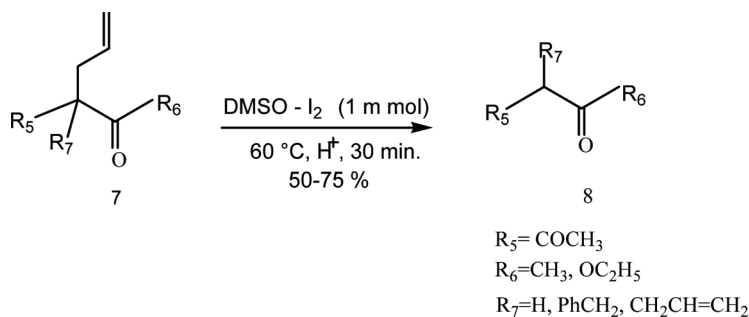
Scheme 4. C-Allyl cleavage in reactive methylene compounds.
