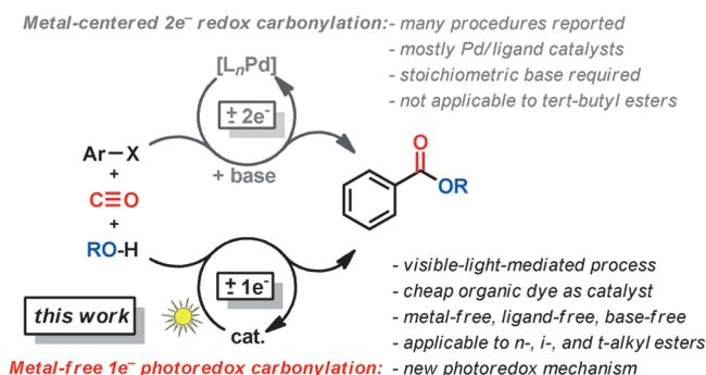
**Scheme 1.** Pd-catalyzed versus photocatalyzed redox carbonylation.
