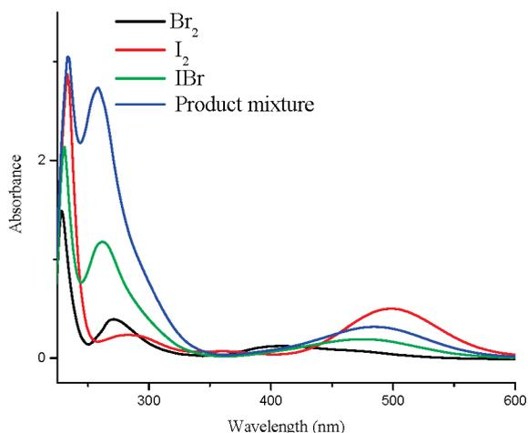
**FIGURE 1.** UV-vis spectra of  $5.54 \times 10^{-4}$  M  $I_2$ ,  $Br_2$ , and  $IBr$  (prepared from  $I_2$  and  $Br_2$ ) in EDC and of diluted product mixture obtained from the reaction (in 25 mL of EDC) of 2-iodo-1-phenylethanol ( $5.54 \times 10^{-3}$  mol) with acid-activated 1:2  $BrO_3^-/Br^-$  (containing  $5.54 \times 10^{-3}$  mol of total Br). The organic layer was diluted 500 times with EDC prior to recording the spectrum.
