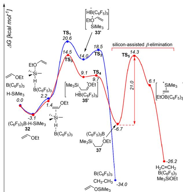
**Figure 2.** DFT calculation of the two possible reaction profiles for ethyl vinyl ether cleavage (ethyl group cleavage (blue) and vinyl group cleavage (red)) in C<sub>6</sub>H<sub>6</sub> using PCM.<sup>16</sup> Gibbs free energies are given in kcal mol<sup>−1</sup> relative to the starting materials.
