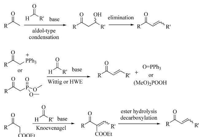
Scheme 1. Standard approaches for the synthesis of  $\alpha,\beta$  unsaturated ketones.
