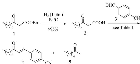
Scheme 2. Preparation of  $\alpha,\beta$ -unsaturated ketone **4**.
