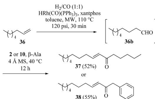
Scheme 3. Telescoped hydroformylation/Verley–Doebner Knoevenagel reaction.
