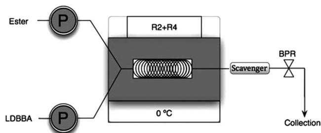
Figure 1. Experimental set up of the flow system.
