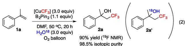
presence of a large excess of H<sub>2</sub><sup>18</sup>O, the corresponding <sup>18</sup>O-labeled product **2a'** was essentially undetected by mass spectrometry. Instead, unlabeled product **2a** was obtained in similar yields as before (cf. Table 1, entries 4 and 13) with 98.5% isotopic purity, therefore ruling out the possibility of water participating in the reaction pathway.
