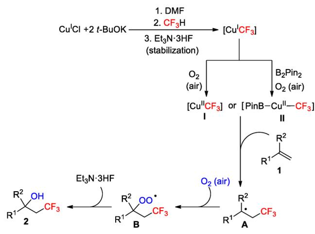
should not be completely ruled out.<sup>17</sup> The radical intermediate **A** is further captured by O<sub>2</sub> from air to form the peroxide radical **B** (cf. eq 2).<sup>6d,18</sup> Finally, the β-trifluoromethyl alcohol product **2** is obtained upon hydrogen abstraction and reduction by Et<sub>3</sub>N·3HF.<sup>6d</sup>
