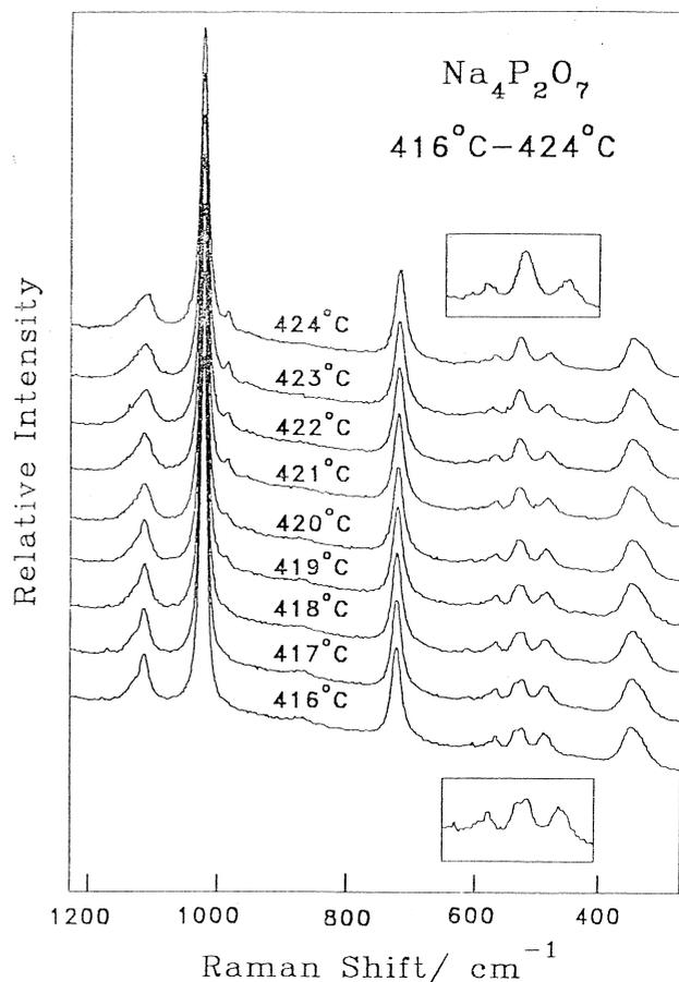
Fig. 5. Thermo-Raman spectra of  $\text{Na}_4\text{P}_2\text{O}_7$  measured in the temperature interval from 416 to 424 °C corresponding to the transformation from  $\epsilon$ -pretransitional phase to  $\delta$ -phase.
