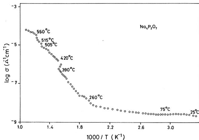
Fig. 2. Temperature dependence conductivity of Na<sub>4</sub>P<sub>2</sub>O<sub>7</sub>.
