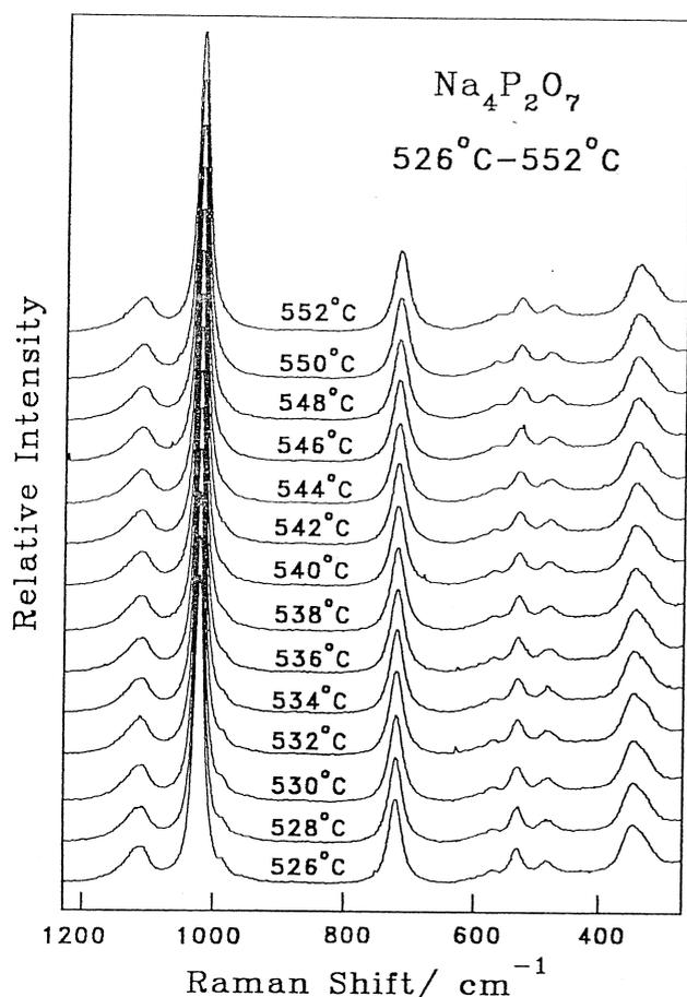
Fig. 6. Thermo-Raman spectra of  $\text{Na}_4\text{P}_2\text{O}_7$  measured in the temperature interval from 526 to 552 °C corresponding to the transformation from  $\beta$ -phase to  $\alpha$ -phase.
