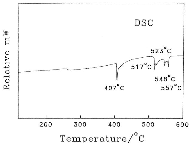
Fig. 1. DSC thermogram of Na<sub>4</sub>P<sub>2</sub>O<sub>7</sub>.
