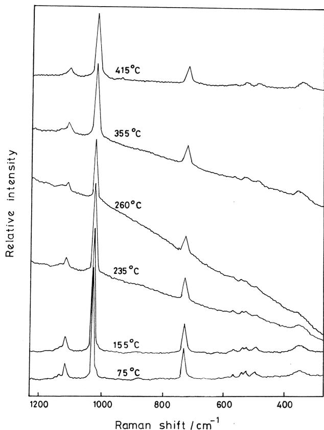
Fig. 4. Thermo-Raman spectra of  $\text{Na}_4\text{P}_2\text{O}_7$  measured in the temperature interval from 75 to 415 °C corresponding to the transformation from  $\epsilon$ -phase to  $\epsilon$ -pretransitional phase.
