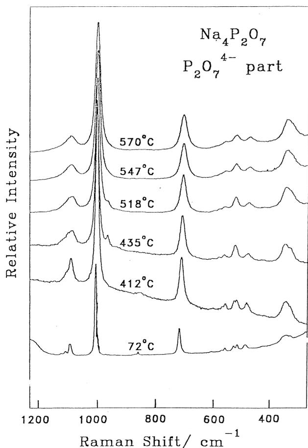
Fig. 3. Typical thermo-Raman spectra of  $\text{Na}_4\text{P}_2\text{O}_7$ .
