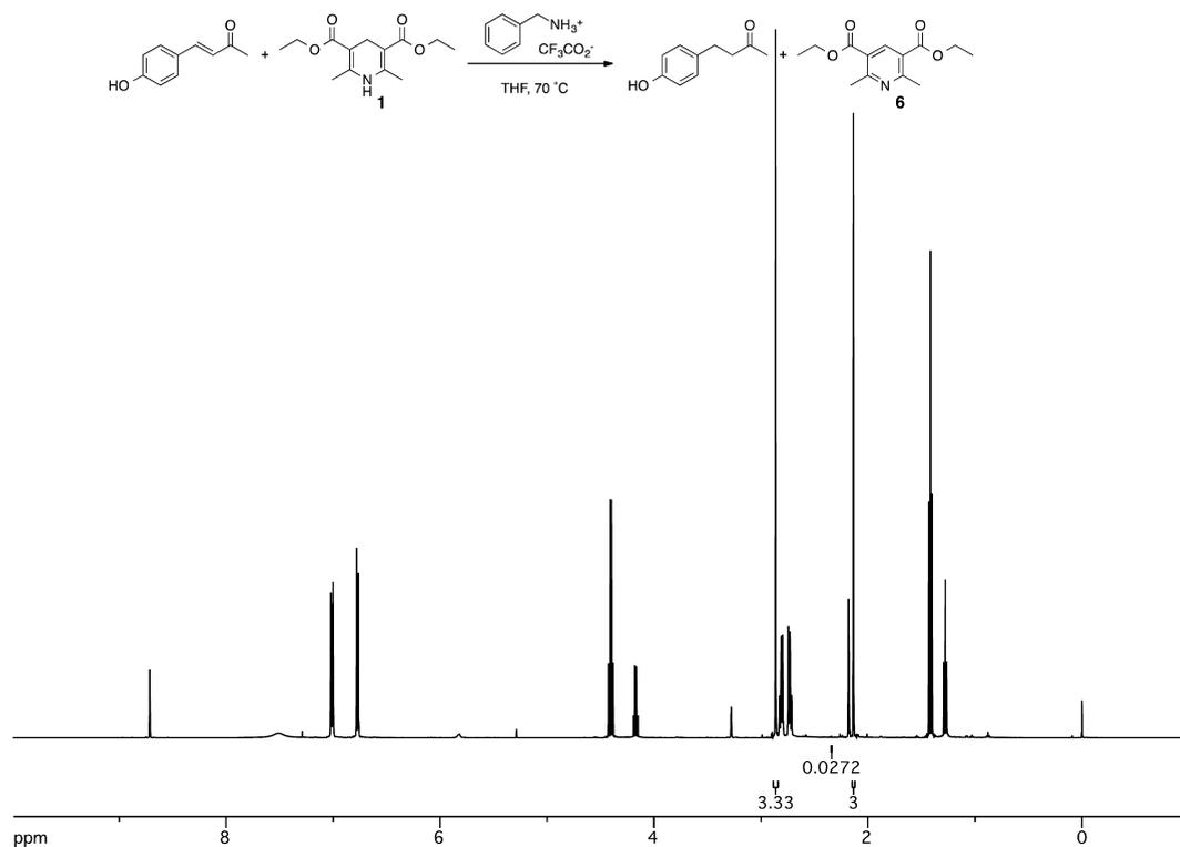
**Figure 2.** Extent of transfer hydrogenation of 4-(4'-hydroxyphenyl)but-3-en-2-one by Hantzsch bis(ethyl ester) and the persistence of Hantzsch materials (1 and 6) after extraction and filtration through a 0.5 cm silica plug.
