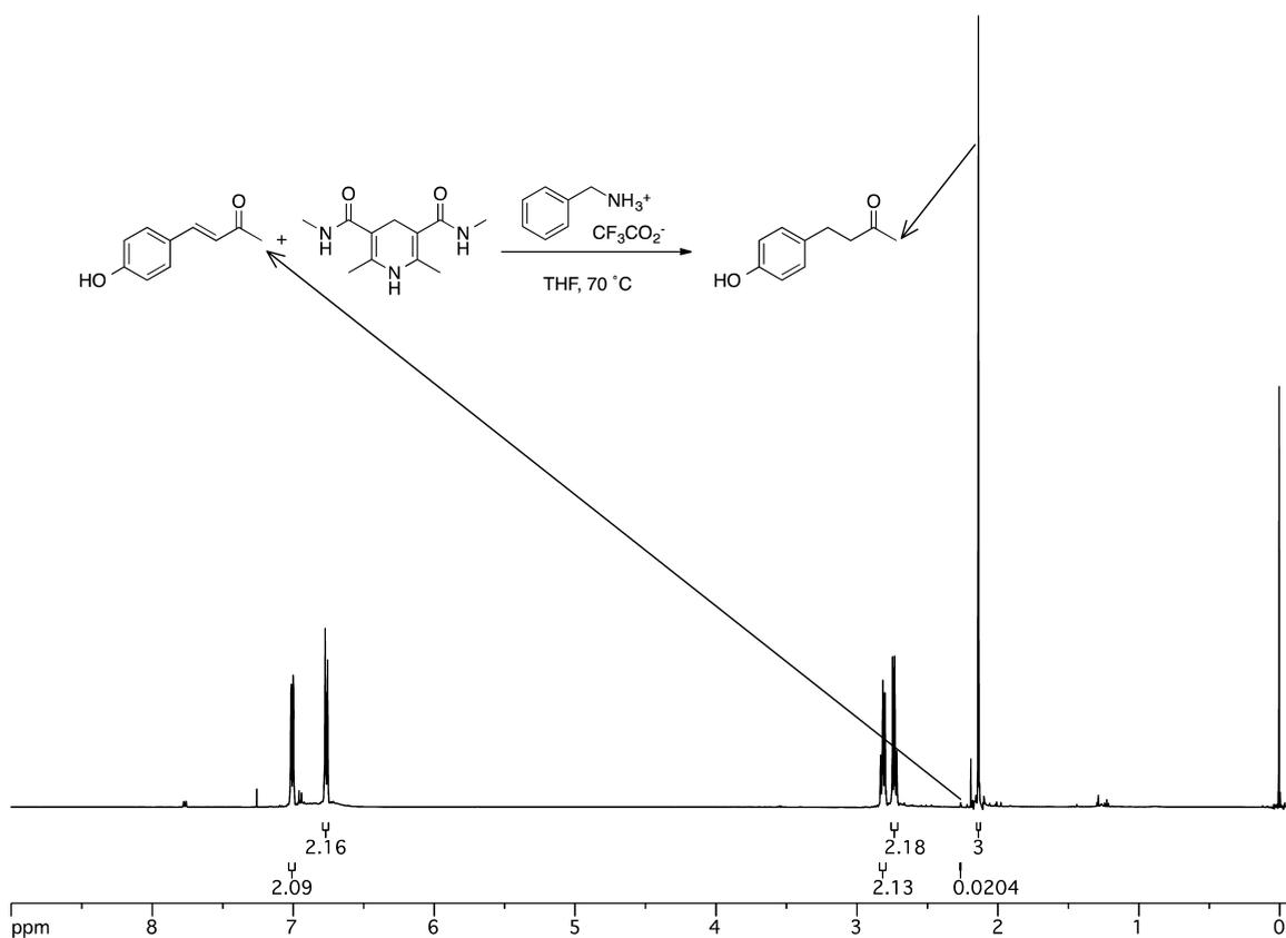
**Figure 1.** Extent of transfer hydrogenation of 4-(4'-hydroxyphenyl)but-3-en-2-one by Hantzsch bis-methylamide and the removal of Hantzsch materials (2 and 3) after extraction and filtration through a 0.5 cm silica plug.
