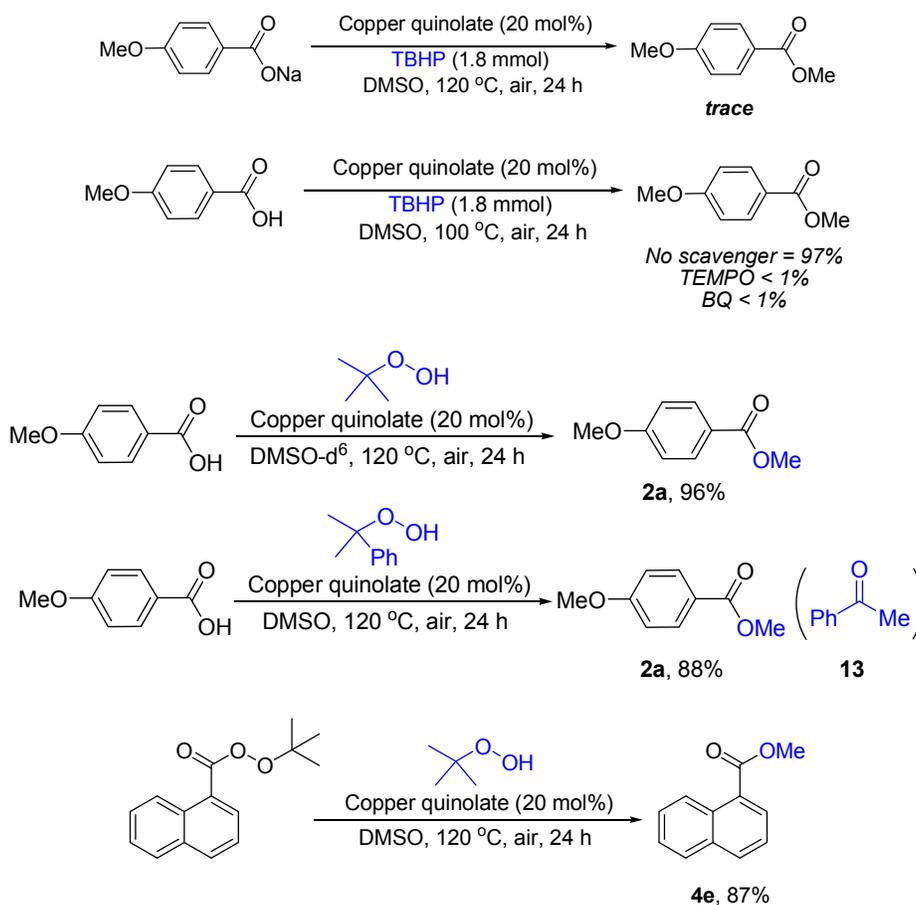
**SCHEME 4. Control experiments and effect of radical inhibitor.**
