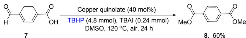
**SCHEME 2. Copper-catalyzed methyl esterification of 4-formylbenzoic acid.**
