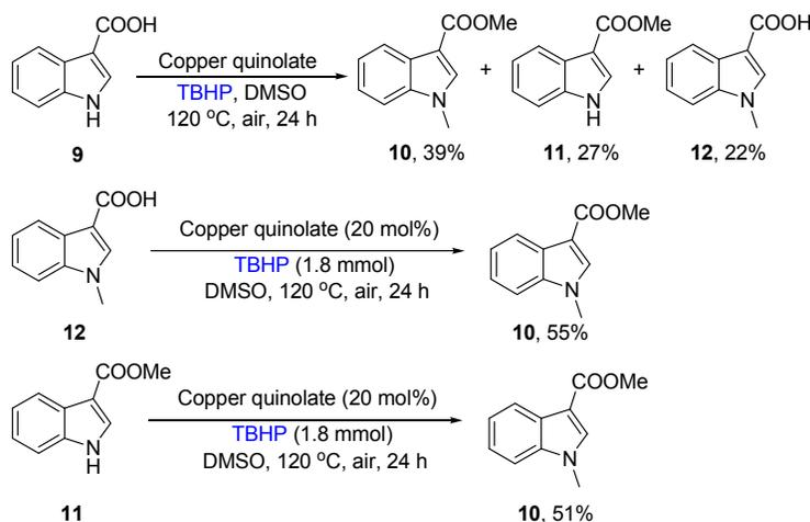
**SCHEME 3. Copper-catalyzed methylation or methyl esterification of 1*H*-indole-3-carboxylic acid or its methyl ester.**
