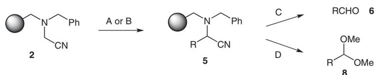
A: a) LDA (5 equiv), THF,  $-70^{\circ}\text{C}$ , 2 h; b) electrophile **4** (15 equiv), 6 h; c) aq.  $\text{NH}_4\text{Cl}$  then wash
