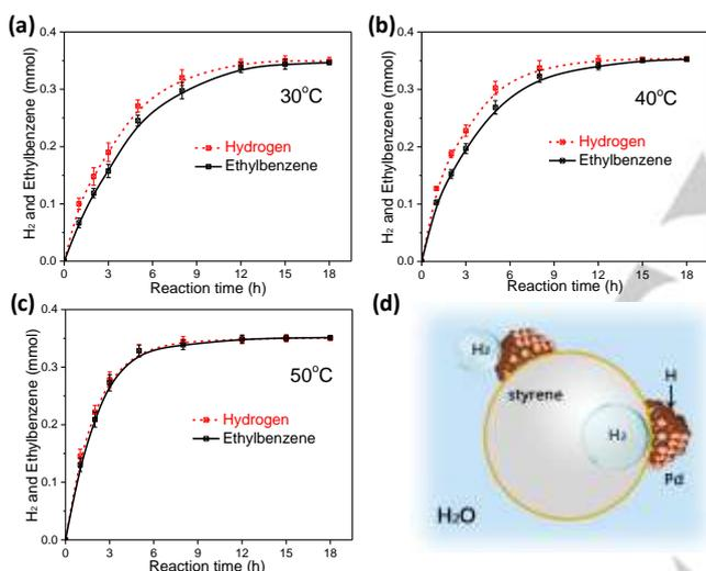
**Figure 3.** Kinetic study of hydrogen evolution and hydrogenation reaction at (a) 30 °C, (b) 40 °C, and (c) 50 °C. (d) Schematic demonstration of the hydrogen buffer effect of the Pd/g-C<sub>3</sub>N<sub>4</sub> Pickering system. Pd NPs are enlarged for better visualization.
