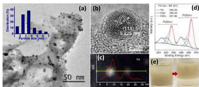
**Figure 1.** Characterizations of 2 wt% Pd/g-C<sub>3</sub>N<sub>4</sub>: (a) TEM image and size distribution, (b) HRTEM image, (c) elemental line profile of Pd, and (d) XPS spectrum of Pd 3d<sub>3/2</sub> and 3d<sub>5/2</sub> orbitals. (e) Photograph of styrene-water Pickering emulsion stabilized by 2wt% Pd/g-C<sub>3</sub>N<sub>4</sub> before (left) and after (right) emulsifying.
