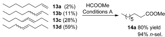
**Scheme 2.** Palladium-catalyzed alkoxy carbonylation of octene mixture.
