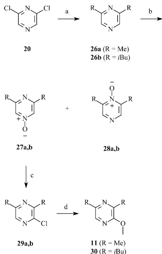
Scheme 2. Synthesis of **11** and **30**: a) RMgBr, Fe(acac)<sub>3</sub>, THF, NMP, 0 °C; b) NaBO<sub>2</sub>·H<sub>2</sub>O<sub>2</sub>·3H<sub>2</sub>O, AcOH, 80 °C; c) POCl<sub>3</sub>, reflux; d) NaOMe, MeOH, 120 °C.
