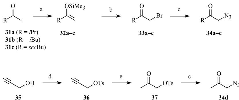
Scheme 3. Synthesis of **34a-d**: a) LDA, Me<sub>3</sub>SiCl, THF, -90 °C; b) Br<sub>2</sub>, pentane, -78 °C; c) NaN<sub>3</sub>, AcOH, EtOH, H<sub>2</sub>O, 0 °C; d) KOH, *p*-TsCl, Et<sub>2</sub>O, 0 °C; e) HgSO<sub>4</sub>, H<sub>2</sub>SO<sub>4</sub>, MeOH, H<sub>2</sub>O, 60 °C.
