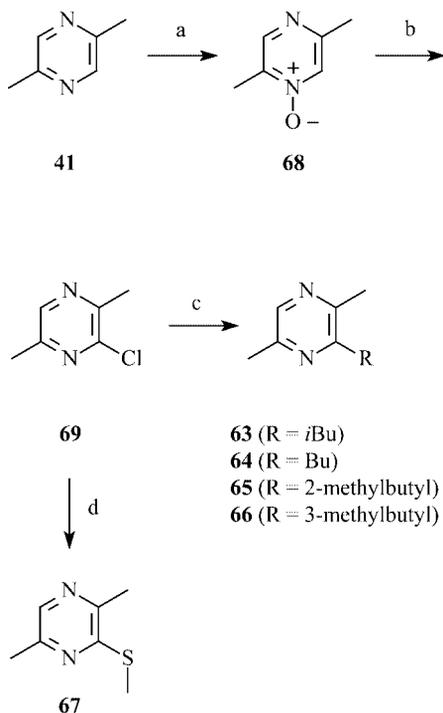
Scheme 6. Synthesis of **63–66** and **67**: a) NaBO<sub>2</sub>·H<sub>2</sub>O<sub>2</sub>·3H<sub>2</sub>O, AcOH, 80 °C; b) POCl<sub>3</sub>, reflux; c) RMgBr, Fe(acac)<sub>3</sub>, THF, NMP, 0 °C; d) NaSMe, DME, 150 °C.
