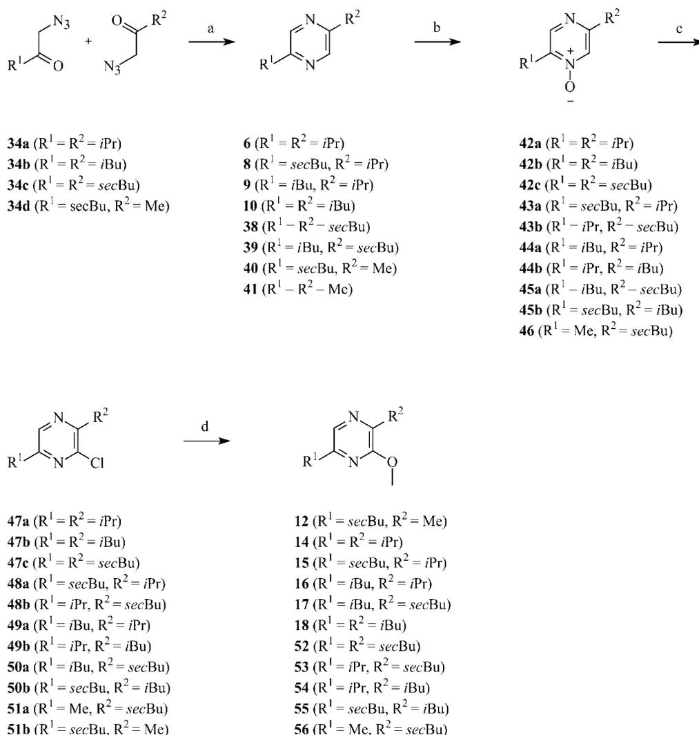
Scheme 4. Synthesis of 2,5-dialkyl-3-methoxypyrazines: a)  $PPh_3$ , benzene,  $20^\circ C$ ; b)  $NaBO_2 \cdot H_2O_2 \cdot 3H_2O$ , AcOH,  $80^\circ C$ ; c)  $POCl_3$ , reflux; d) NaOMe, MeOH,  $120^\circ C$ .
