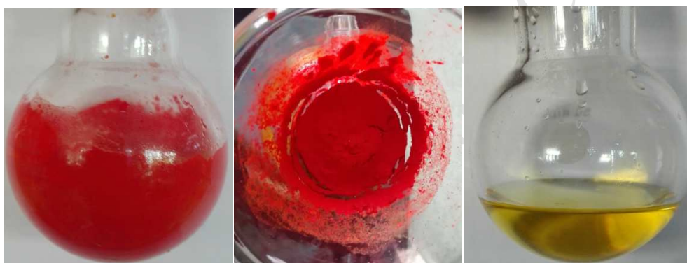
(d) Reaction mixture (after reaction); (e) The product isolated by direct filtration; (f) The recovered IL9 in aqueous.
