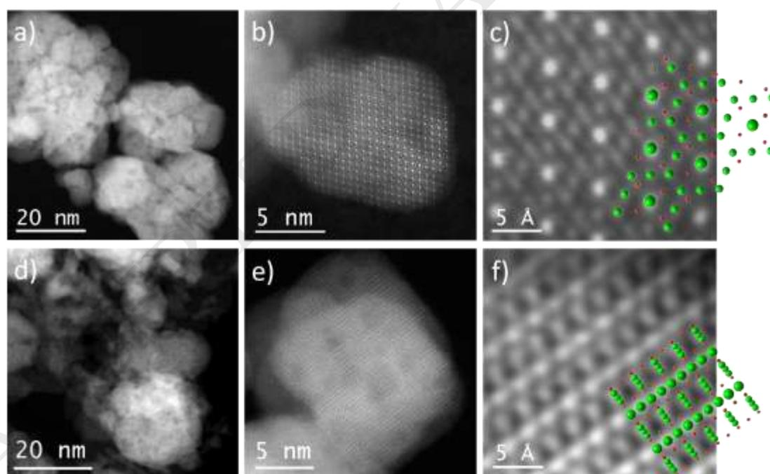
**Figure 7.**  $C_s$ -corrected STEM-HAADF data. a) Low-magnification image showing several Mn-ST nanoparticles. b) High-resolution image of a Mn-ST isolated nanoparticle along the [111] zone axis. c) A closer look of the structure of the Mn-ST nanoparticle with the model superimposed. d) Low-magnification image of Mn-HT material. e) An isolated  $Mn_3O_4$ -HT nanoparticle along the [011]
