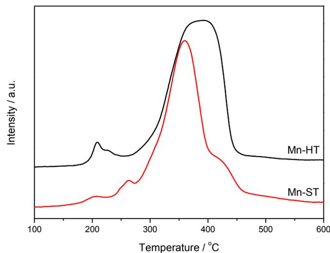
**Figure 6.** H<sub>2</sub>-TPR for the manganese oxide catalysts.
