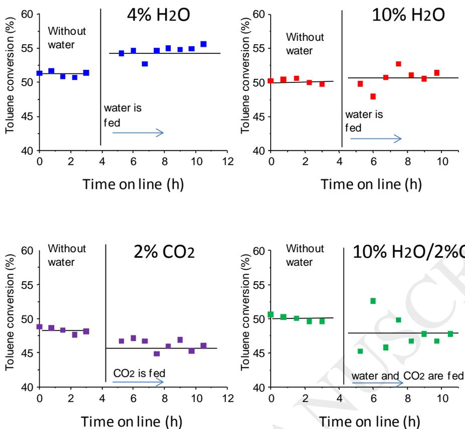
**Figure 2. Toluene conversion under different reaction feeds. Toluene concentration: 200 ppm. Reaction temperature: 125 °C. GHSV: 6000 h<sup>-1</sup>.**
