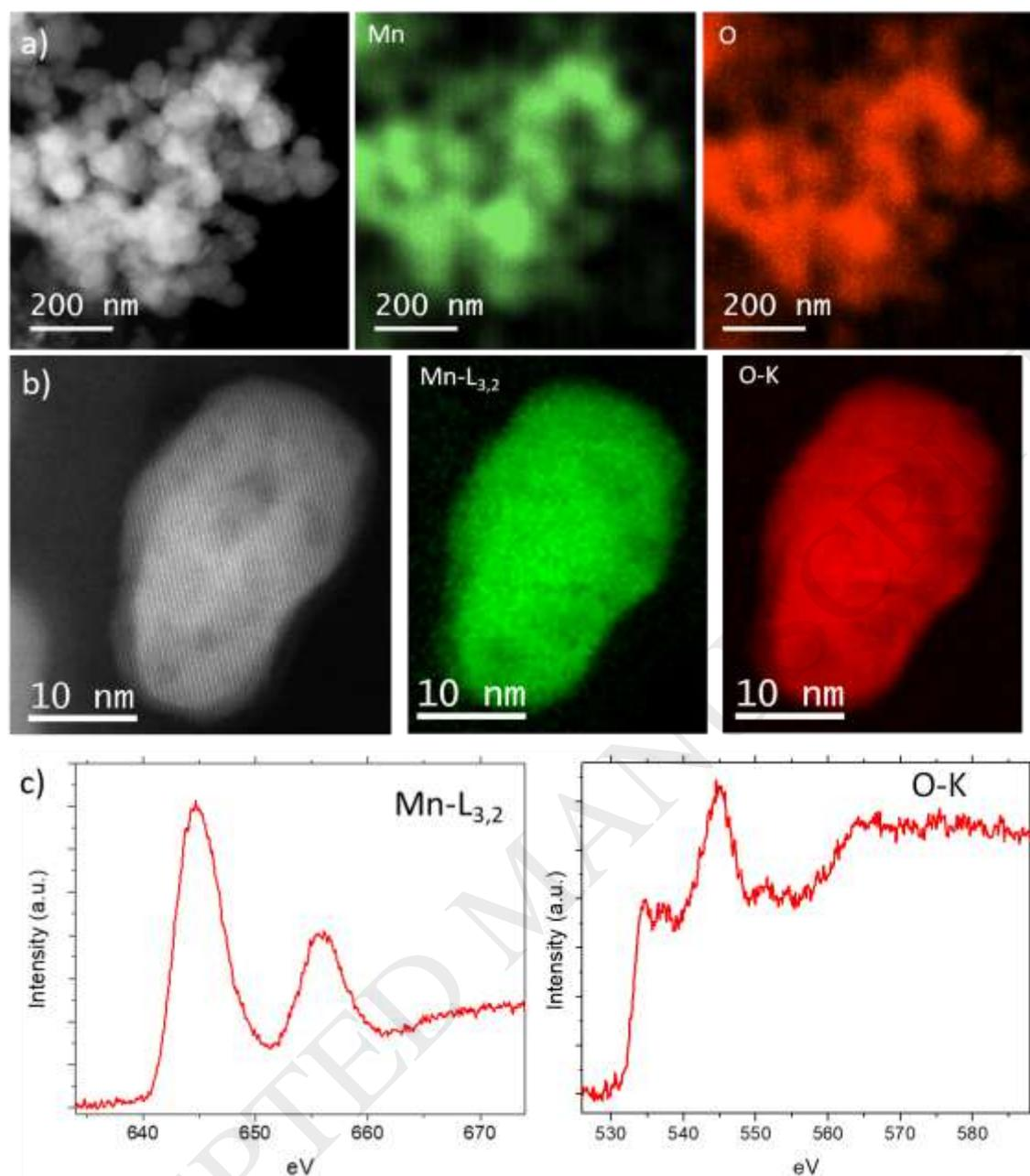
**Figure 8.** Study by TEM of Mn-HT catalyst. a) EDS mapping analysis of several nanoparticles which confirms the presence of Mn (green map) and O (red map). b) EEL spectrum image of a Mn-HT nanoparticle showing the perfect concordance between the Mn and O. c) EEL spectra of the signals extracted corresponding to Mn and O edges respectively.
