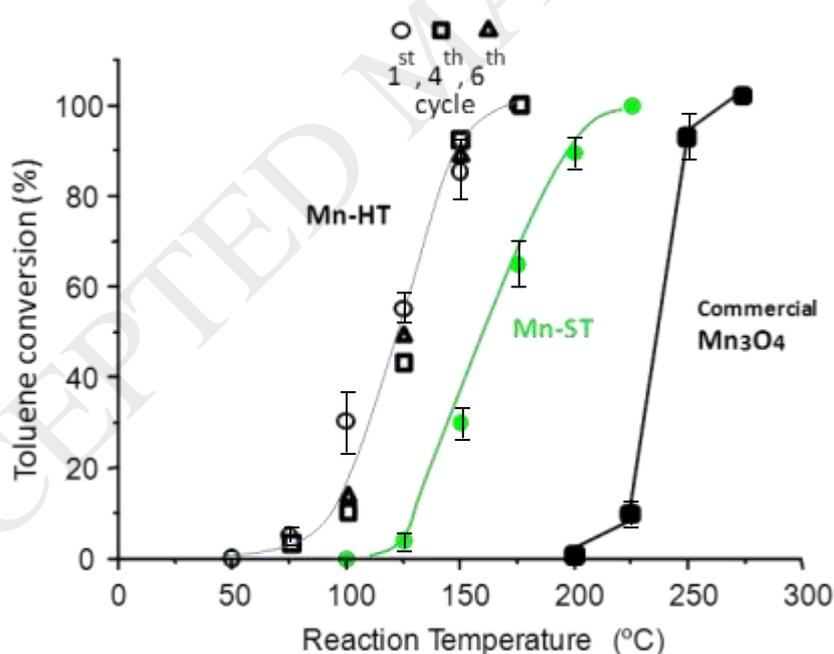
Figure 1. Variation of the toluene conversion with the reaction temperature for manganese oxide catalysts. 200 ppm in synthetic air. GHSV = 6000 h<sup>-1</sup>.
