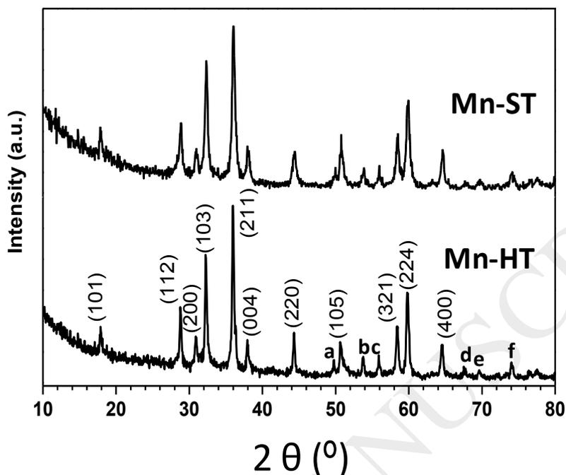
**Figure 4.** XRD patterns of manganese oxide catalysts. In both cases the only phase detected is  $\text{Mn}_3\text{O}_4$ . The small diffractions a, b, c, d, e and f correspond to (204), (312), (303), (402), (305) and (413), respectively.
