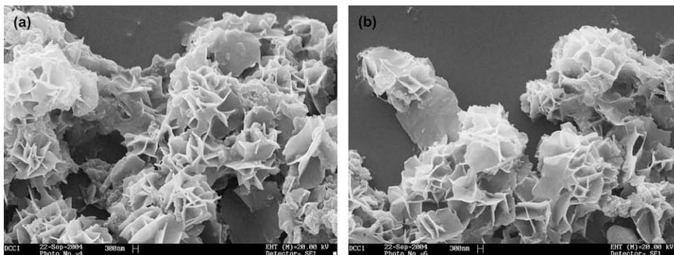
Figure 1. SEM images of the co-polymers CM8-3 (a), CM8-4 (b).
