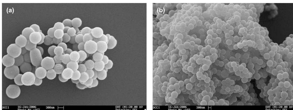
Figure 2. SEM images of the co-polymer C8.
