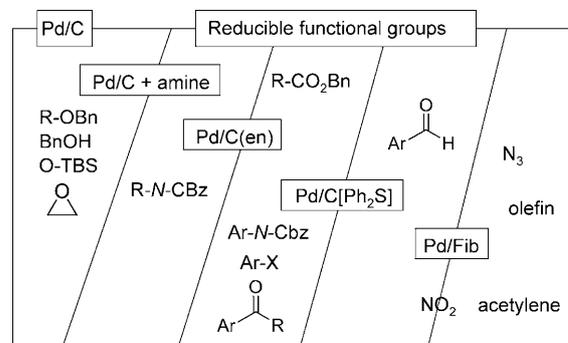
**Figure 1.** Pd-catalyzed chemoselective hydrogenation with combination of various catalytic poisons.
