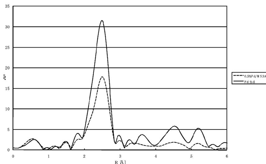
Figure 3. Pd K-edge K<sup>3</sup>χ(k) EXAFS Fourier transforms of 0.5% Pd/MS3A and Pd foil.
