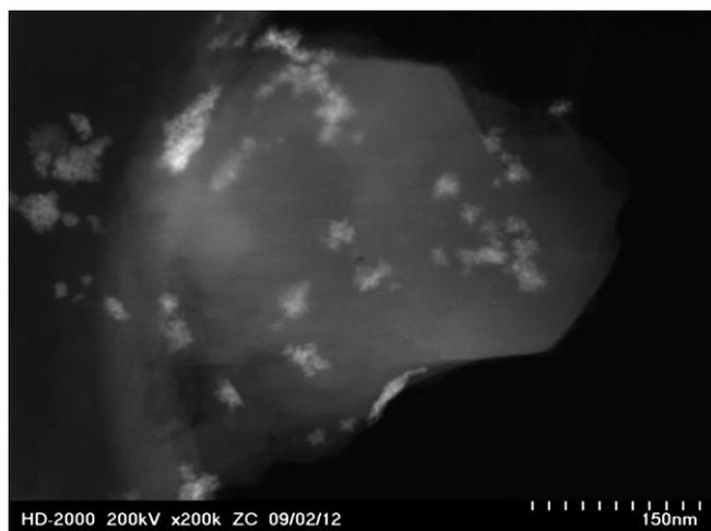
Figure 2. STEM of 0.5% Pd/MS3A.
