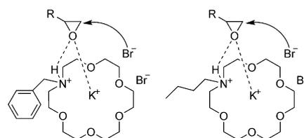
Scheme 1. The coupling reaction of  $\text{CO}_2$  and epoxide catalyzed by aza-crown ether complex cation ionic liquid.
