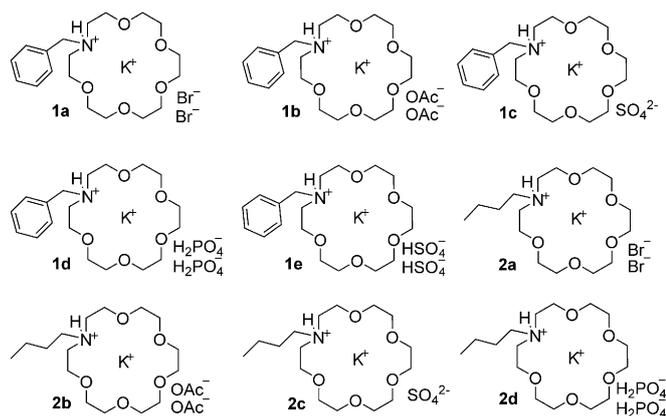
Figure 1. The structures of aza-crown ether complex cation ionic liquids.
