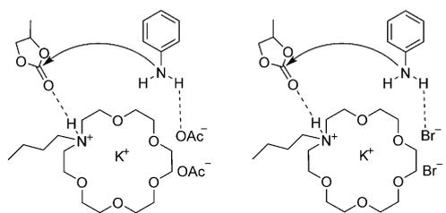
**Scheme 2.** The model of aza-crown ether complex cation ionic liquids to activate substrates.
