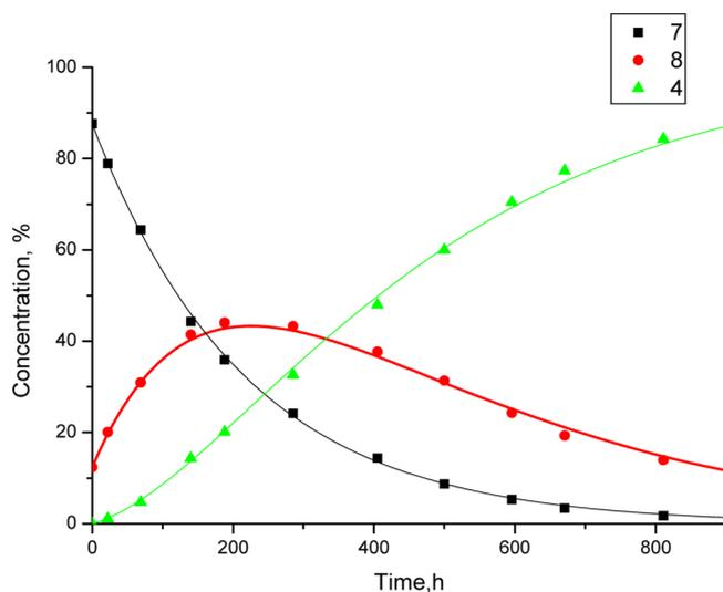
**Figure 3.**  $^{31}\text{P}\{^1\text{H}\}$  NMR monitoring of the rearrangement of 7 to 8 and formation of 4. Dots correspond to the experimental points and continuous lines to the simulated curves.
