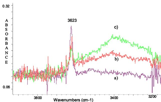
**Figure 4.** IR spectra in the ν(OH) region in hexane solution: (a) <sup>t</sup>BuOH (*c* = 0.04 M); b) <sup>t</sup>BuOH in the same concentration in the presence of **6**; c) the same mixture as in (b) at 0 °C.
