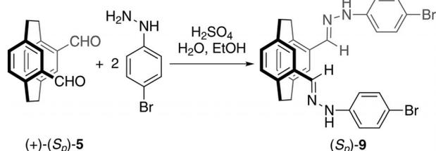
Scheme 5. Synthesis of (*S<sub>p</sub>*)-(4-bromophenyl)hydrazone **9** from enantiopure (+)-(*S<sub>p</sub>*)-**5**.
