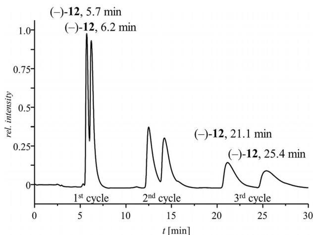
Figure 2. Chromatographic resolution of *rac*-**12** by analytical HPLC on an analytical chiral CHIRALPAK IA phase (*n*-hexane/dichloromethane, 90:10 v/v; flow rate 1.5 mL min<sup>-1</sup>).
