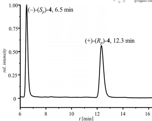
Figure 1. Chromatographic resolution of *rac-4* by analytical HPLC on an analytical chiral CHIRALPAK IA phase (*n*-hexane/ethanol, 75:25 v/v; flow rate 1.0 mL min<sup>−1</sup>).
