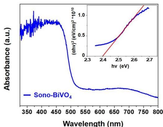
**Figure 3.** UV-visible absorption spectrum and Tauc plot (inset) of Sono-BiVO<sub>4</sub> crystals.
