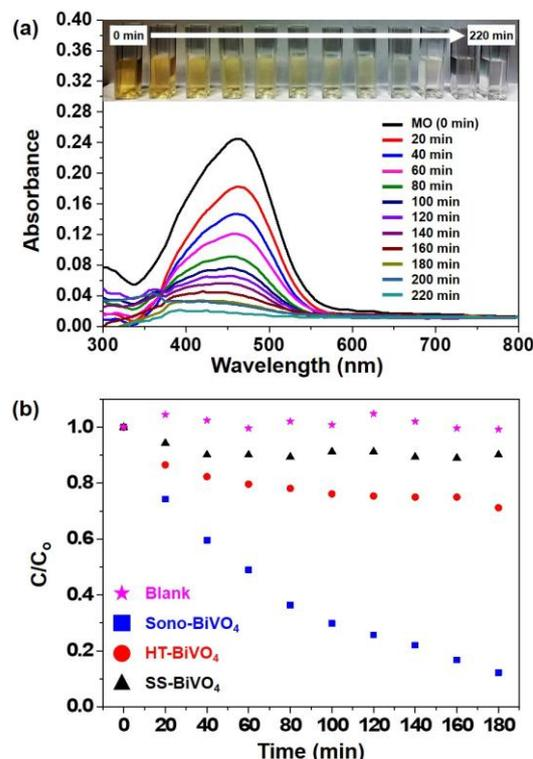
**Figure 4.** (a) Time-dependent UV-Vis absorption spectra of MO solution in the presence of the Sono-BiVO<sub>4</sub> crystals. (b) Photocatalytic degradation rates of MO when using Sono-BiVO<sub>4</sub> (blue squares), HT-BiVO<sub>4</sub> (red circles), SS-BiVO<sub>4</sub> (black triangles) crystals, and without BiVO<sub>4</sub> (pink stars).
