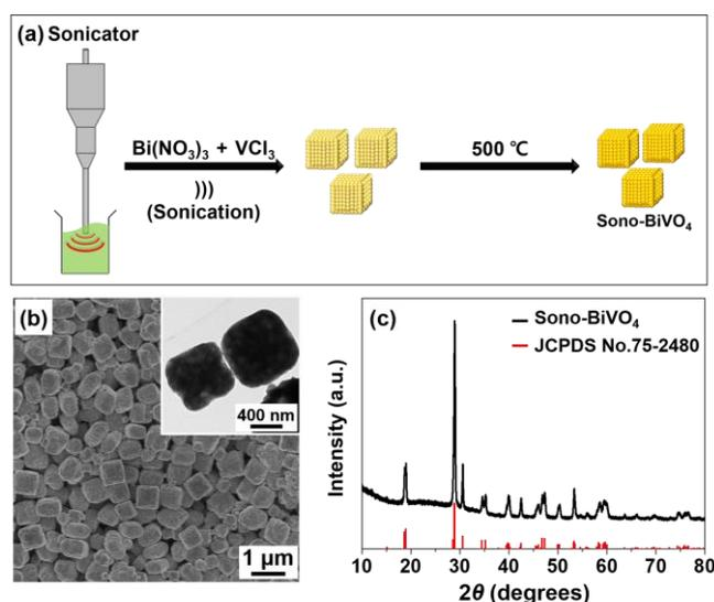
**Figure 2.** (a) Schematic of the preparation of Sono-BiVO<sub>4</sub> crystals. (b) SEM and TEM (inset) images of the Sono-BiVO<sub>4</sub> crystals. (c) XRD pattern of the Sono-BiVO<sub>4</sub> crystals.
