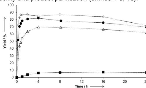
**Figure 1.** Variation of the catalyst loading in the decarboxylation of phenylalanine (**1a**) to 2-phenethylamine (**2a**). Conditions: **1a** (0.25 mmol), isophorone, DMSO (1 mL), 130 °C. The yield of **2a** was determined by GC analysis using benzonitrile as the internal standard. Legend: (■) no catalyst, (△) 1 mol%, (●) 2.5 mol%, and (◇) 5 mol% of isophorone.
