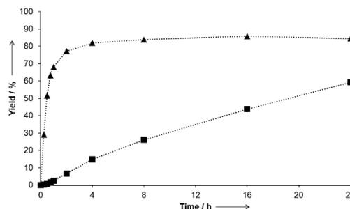
**Figure 3.** Tandem decarboxylation – *N*-formylation of phenylalanine (**1a**, ▲) versus *N*-formylation of 2-phenethylamine (**2a**, ■) in DMF. Conditions: **1a** or **2a** (0.25 mmol), isophorone (0.0125 mmol), DMF (1 mL), 130 °C. The yield of *N*-(2-phenethyl)formamide (**3a**) was determined by GC analysis using benzonitrile as the internal standard.
