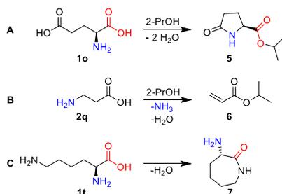
**Scheme 2.** Side reactions observed during the isophorone-catalysed decarboxylation of certain amino acids: [A] lactamisation and esterification of glutamic acid (**1o**) to an alkyl pyroglutamate (**5**); [B] deamination and esterification of  $\beta$ -alanine (**2q**) to an alkyl acrylate (**6**), and [C] lactamisation of lysine (**1t**) to  $\alpha$ -amino- $\epsilon$ -caprolactam (**7**).
