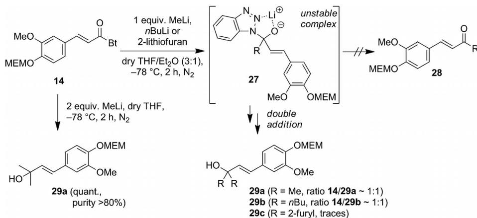
Scheme 8. Reaction of MEM-protected *N*-feruloylbenzotriazole **14** with alkyllithium reagents gave the corresponding tertiary alcohols **29a–29c**.
