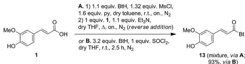
Scheme 2. Synthesis of *N*-feruloylbenzotriazole (**13**).
