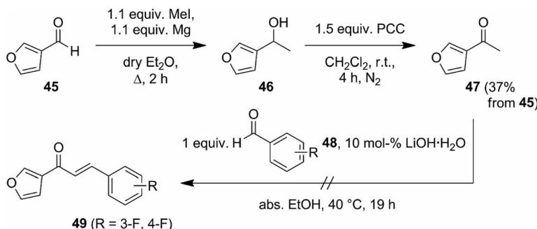
Scheme 13. Aldol reaction of 3-acetylfuran **47** is not a straightforward route to 3-furyl-chalcones; PCC = pyridinium chlorochromate.
