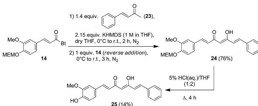
Scheme 6. Conversion of MEM-protected *N*-feruloylbenzotriazole **14** into curcuminoids **24** and **25**; KHMDS = potassium hexamethylsilazide.
