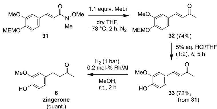
Scheme 10. Illustration of the use of MEM-protected *N*-feruloyl-substituted Weinreb amide **31** for the synthesis of ketones: preparation of zingerone (**6**).
