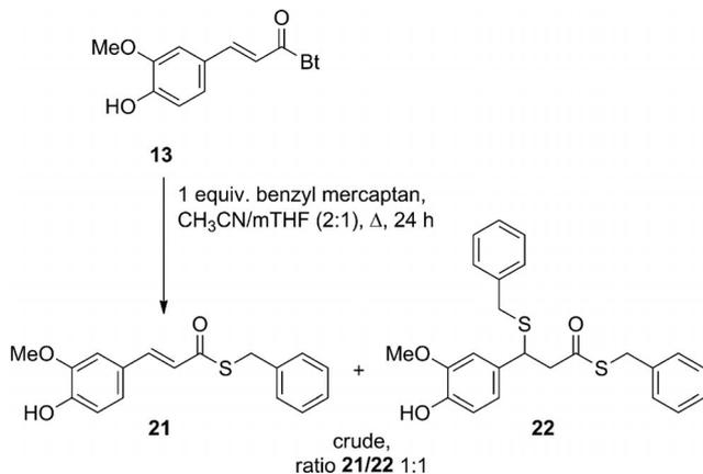
Scheme 5. *N*-Feruloylbenzotriazole (**13**) behaves as an ambident electrophile towards benzyl mercaptan; mTHF = 2-methyltetrahydrofuran.
