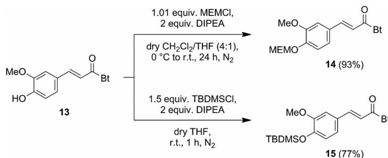
Scheme 3. Preparation of MEM- and TBDMS-protected *N*-feruloylbenzotriazoles **14** and **15**; DIPEA = diisopropylethylamine.
