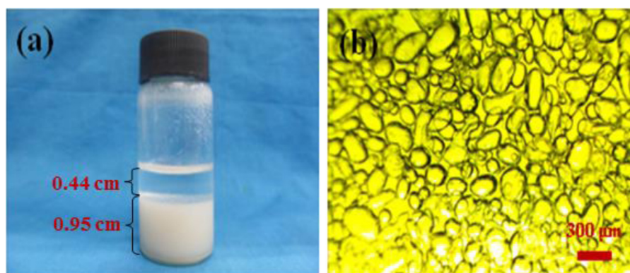
Fig. 2. (a) The digital photograph and (b) the corresponding optical microscopy image of \text{SiO}_2\text{—Me\&SO}_3\text{H} NPs-stabilized Pickering emulsions.
