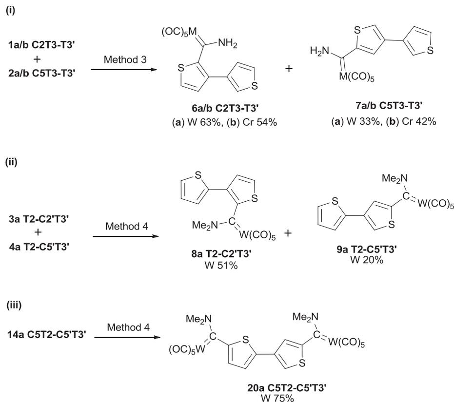
**Scheme 2.** Aminolysis of mono-ethoxycarbene complexes **Method 3**: Adding an ether solution saturated with  $\text{NH}_3(\text{g})$ ; **Method 4**: The *in situ* generation of  $\text{NHMe}_2$  from  $[\text{NH}_2\text{Me}_2]\text{Cl}$  and  $\text{NaOH}$  in an aqueous THF solution.
