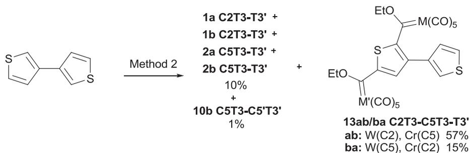
**Scheme 3.** Mixed metal biscarbene complexes from 3,3'-bithienyl substrates. **Method 2:** 1 eq  $n$ -BuLi, 1 eq  $M(\text{CO})_6$  in THF, 1 eq  $n$ -BuLi, 1 eq  $M'(\text{CO})_6$  in THF, 2 eq  $[\text{Et}_3\text{O}][\text{BF}_4]$  in DCM.
