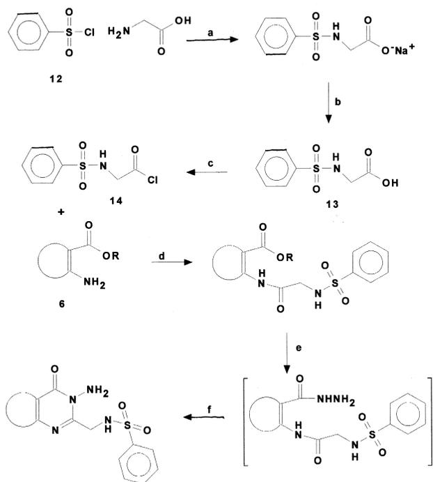
**Figure 2.** Synthesis of sulphonamido derivatives (**10g**, **h**, **o**, **v** and **w**).
