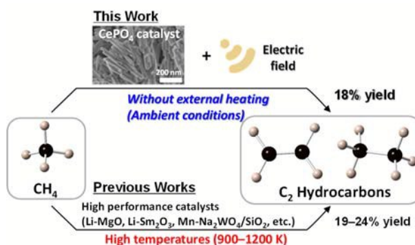
Scheme 1. Low-temperature OCM by a monoclinic CePO 4 nanorod catalyst combined with an electric field.
