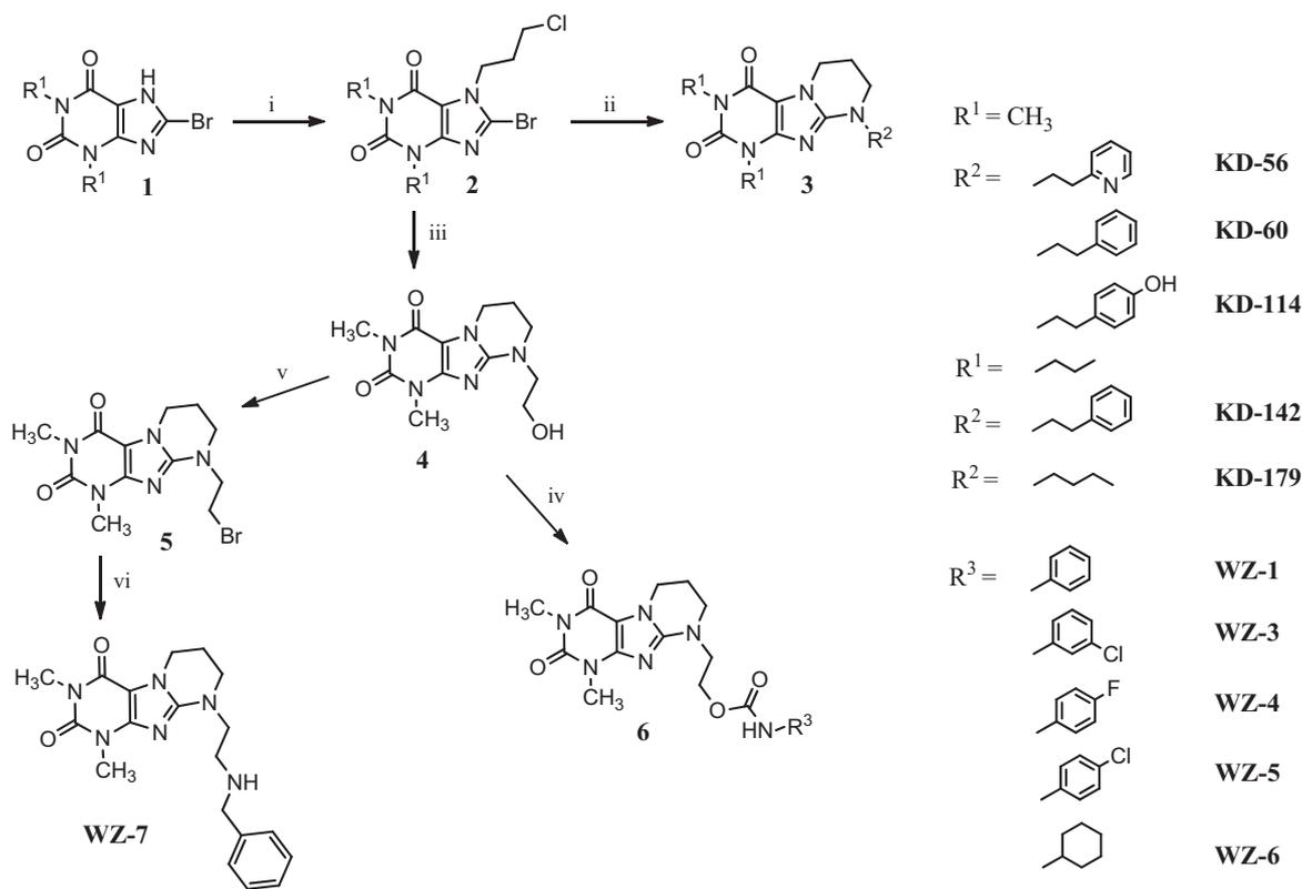
(i) Cl(CH<sub>2</sub>)<sub>3</sub>Br (ii) R<sup>2</sup>NH<sub>2</sub> (iii) NH<sub>2</sub>(CH<sub>2</sub>)<sub>2</sub>OH (iv) R<sup>3</sup>NCO (v) PBr<sub>3</sub> (vi) PhCH<sub>2</sub>NH<sub>2</sub>
