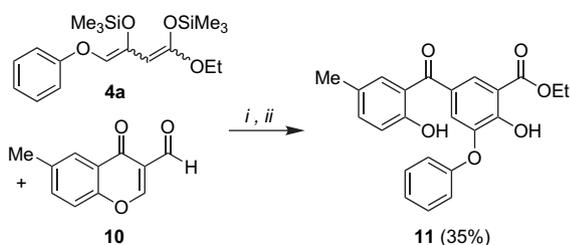
Scheme 5. Synthesis of **11**: (i)  $\text{Me}_3\text{SiOTf}$  (0.3 equiv), 20 °C, 10 min; (ii) (1) **4a** (1.3 equiv),  $\text{CH}_2\text{Cl}_2$ , 0  $\rightarrow$  20 °C, 12 h; (2) HCl (10%).
