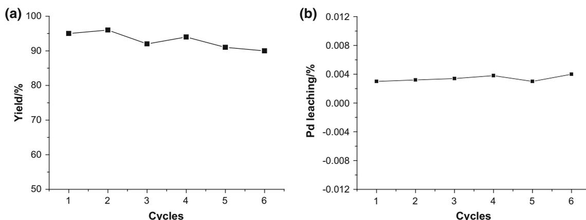
**Fig. 5** Yield (a) and Pd leaching (b) for Pd<sub>63</sub>Sn<sub>37</sub>/C NPs in Heck reaction of bromobenzene with styrene
