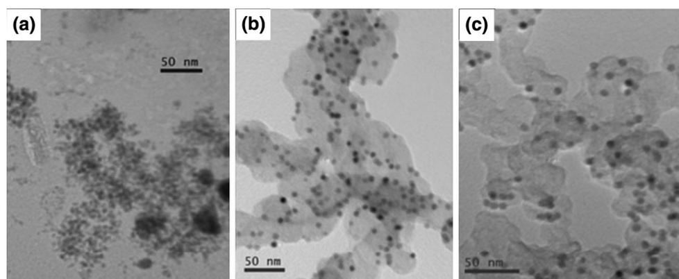
**Fig. 4** TEM images of unsupported Pd<sub>63</sub>Sn<sub>37</sub> NPs after Heck reaction (a), Pd<sub>63</sub>Sn<sub>37</sub>/C NPs after one cycle (b) and Pd<sub>63</sub>Sn<sub>37</sub>/C NPs after six cycles (c)
