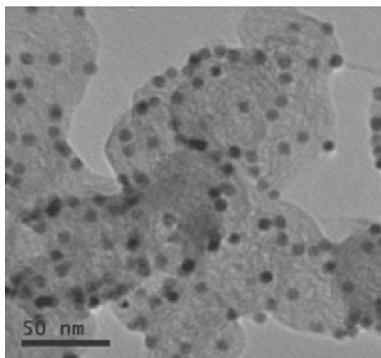
**Fig. 2** TEM images of Pd<sub>63</sub>Sn<sub>37</sub>/C NPs before catalytic reaction
