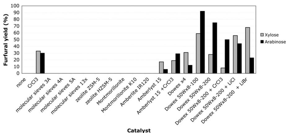
Fig. 5. Dehydration of xylose and arabinose in IL solution with different heterogeneous catalysts.
