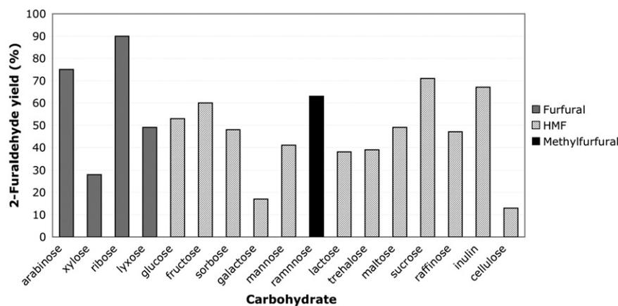
Fig. 6. Dehydration of carbohydrates with Dowex® 50Wx8-200 ion exchange resin.
