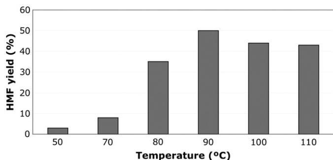
Fig. 3. HMF yields as a function of temperature using Dowex® 50Wx8-200 as catalyst and glucose as substrate.
