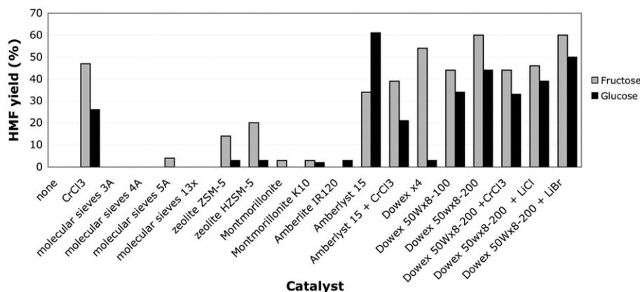
Fig. 2. Dehydration of fructose and glucose in IL solution with different heterogeneous catalysts.
