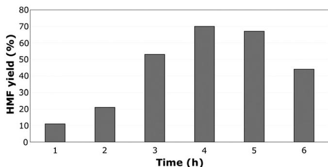
Fig. 4. HMF yields as a function of reaction time using Dowex® 50Wx8-200 as catalyst and glucose as substrate.
