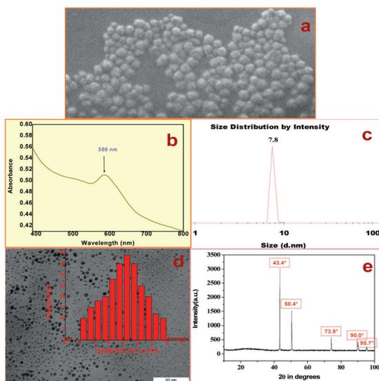
**Fig. 1** (a) SEM image of the cooperative assembly. (b) UV-vis spectrum. (c) DLS data. (d) TEM image. (e) Powder XRD data.
