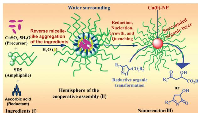
Scheme 1 Fabrication of Cu(0)-NPs and their catalytic activity.
