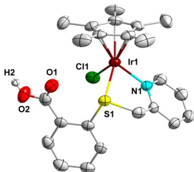
**Figure 3.** Molecular structure of the cation of **3**. Bond lengths (Å): Ir(1)–S(1) 2.3637 (14), Ir(1)–N(1) 2.099(4), Cl(1)–Ir(1) 2.3791(15), Ir–C 2.145(6)–2.194(5). Bond angles (deg): S(1)–Ir(1)–N(1) 81.78(14), S(1)–Ir(1)–Cl(1) 93.44(5), N(1)–Ir(1)–Cl(1) 85.33(13), O(1)–C(7)–O(2) 122.9(7).
