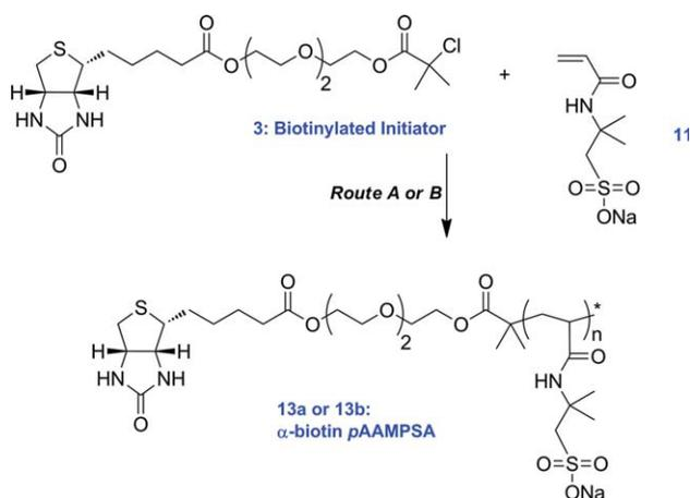
**SCHEME 4** Polymerization of 2-acrylamido-2-methyl-1-propane-sulfonic acid, sodium salt, Route A by LRP *N*-(*n*-ethyl)-2-pyridylmethanimine, CuCl, H<sub>2</sub>O/MeOH/DMSO, 30 °C; Route B by LRP: Me<sub>6</sub>-TREN, CuCl, DMSO, 25 °C. [Color figure can be viewed in the online issue, which is available at [wileyonlinelibrary.com](http://wileyonlinelibrary.com).]
