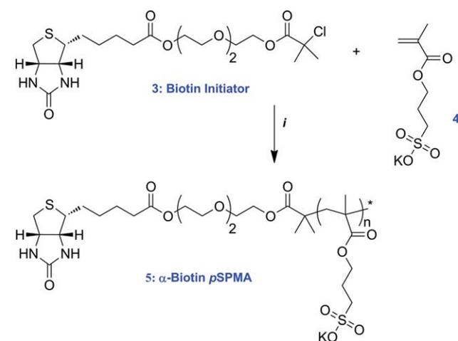
**SCHEME 2** (i) Polymerization of *α*-biotin poly(3-sulfopropylmethacrylate, potassium) by LRP: *N*-(*n*-ethyl)-2-pyridylmethanimine, CuBr, CuBr<sub>2</sub>, H<sub>2</sub>O/MeOH/DMSO, 40 °C. [Color figure can be viewed in the online issue, which is available at [wileyonlinelibrary.com](http://wileyonlinelibrary.com).]
