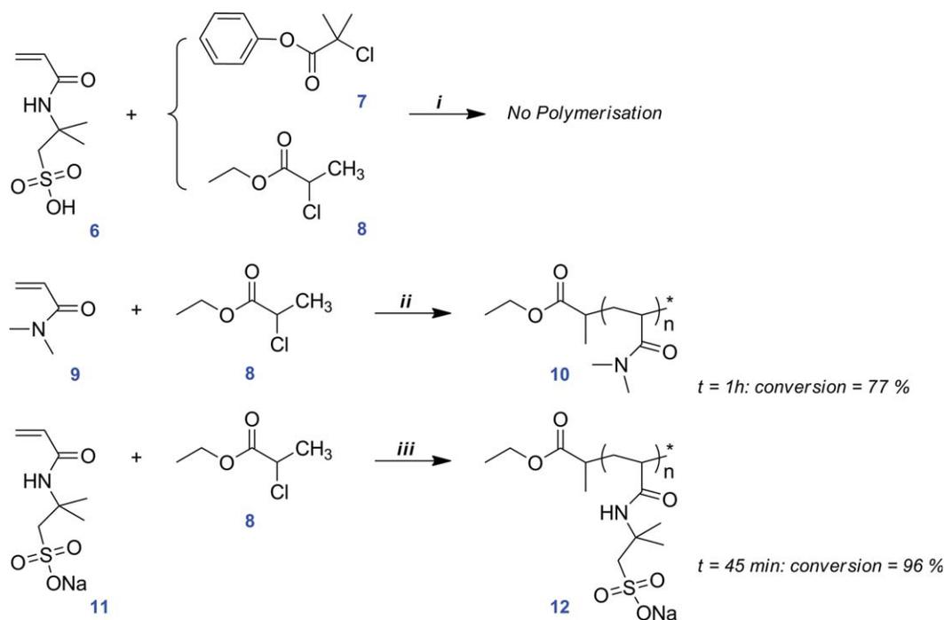
**SCHEME 3** Polymerization tests: (i) Polymerization of 2-acrylamido-2-methyl-1-propanesulfonic acid by LRP: Me<sub>6</sub>-TREN, CuCl, DMSO, 30 °C; (ii) *N,N*-dimethylacrylamide by LRP: Me<sub>6</sub>-TREN, CuCl, DMSO, 30 °C; (iii) 2-acrylamido-2-methyl-1-propanesulfonic acid, sodium salt by LRP: Me<sub>6</sub>-TREN, CuCl, H<sub>2</sub>O/DMSO, 30 °C. [Color figure can be viewed in the online issue, which is available at [wileyonlinelibrary.com](http://www.interscience.wiley.com).]
