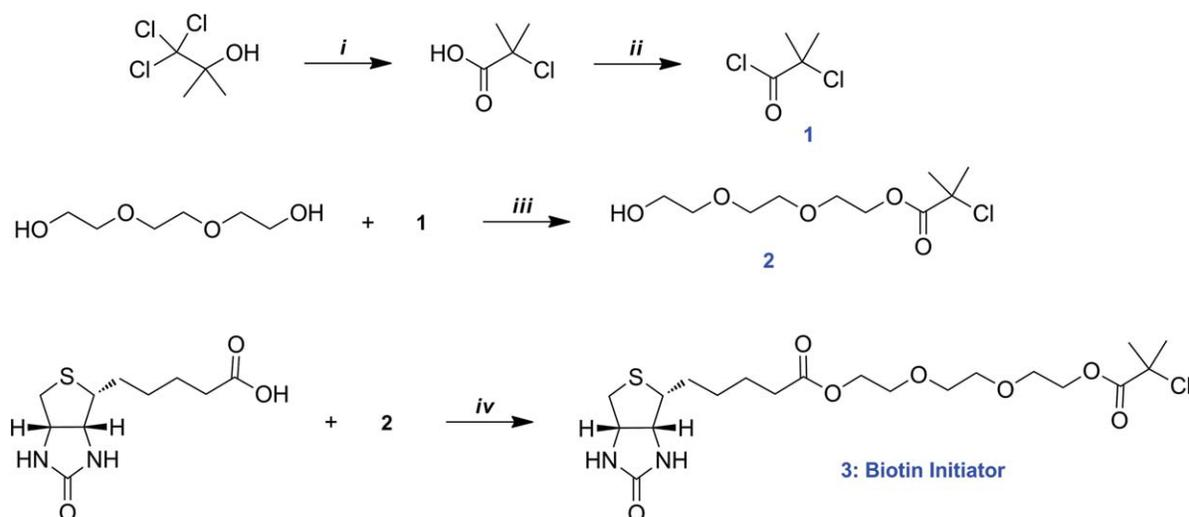
**SCHEME 1** Synthesis of biotin initiator: (i) Kundiger method<sup>32</sup>: H<sub>2</sub>SO<sub>4</sub>, from 0 °C to 25 °C; (ii) SOCl<sub>2</sub>, from 0 °C to 25 °C; (iii) TEA, THF, from 0 °C to 20 °C; (iv) Yamaguchi procedure: TEA, DMF, from 0 °C to 20 °C. [Color figure can be viewed in the online issue, which is available at [wileyonlinelibrary.com](http://wileyonlinelibrary.com).]
