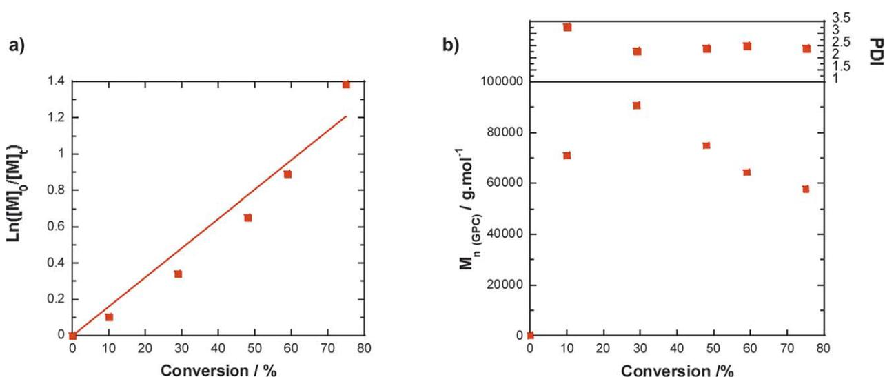
**FIGURE 1** Kinetic plot of pAAMPSA (a) and evolution of  $M_n$  and polydispersity index (PDI) with time (b). Synthesis conditions: Route A by LRP: *N*-(*n*-ethyl)-2-pyridylmethanimine, CuCl, H<sub>2</sub>O/MeOH/DMSO, 30 °C. [Color figure can be viewed in the online issue, which is available at [wileyonlinelibrary.com](http://wileyonlinelibrary.com).]
