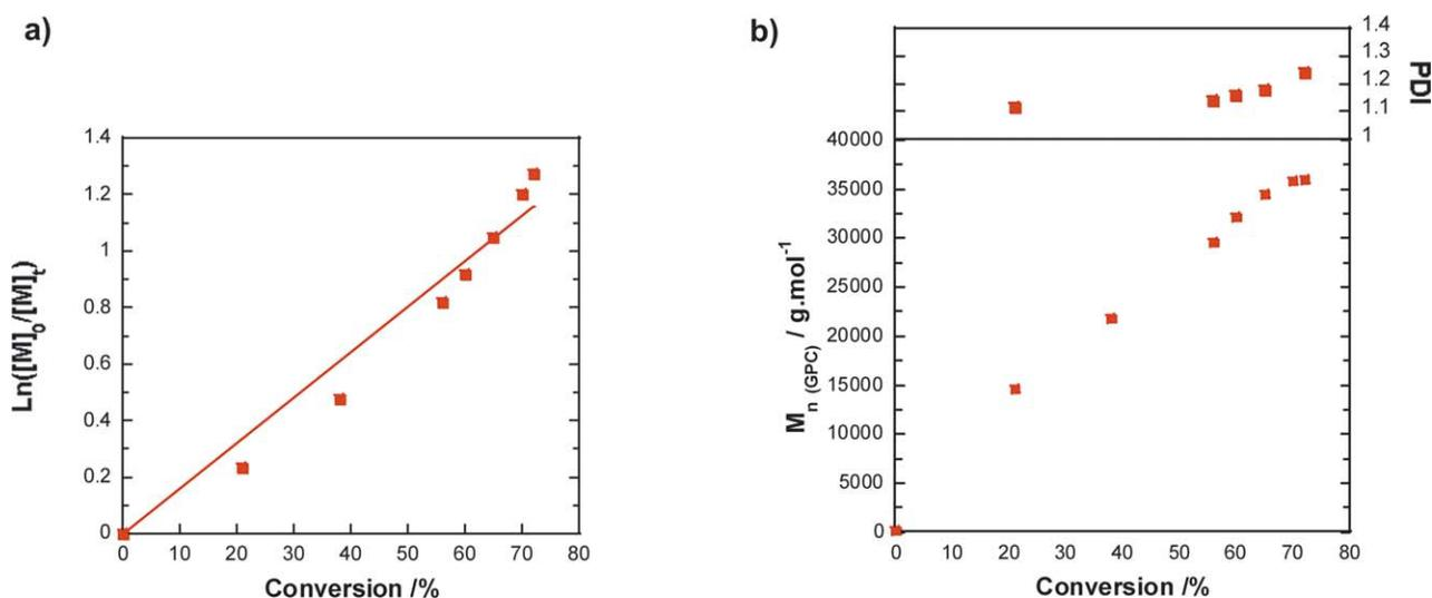
**FIGURE 2** Kinetic plot of *pAAMPSA* (a) and evolution of  $M_n$  and PDI with conversion (b). Synthesis conditions: Route B by LRP:  $\text{Me}_6\text{-TREN}$ ,  $\text{CuCl}$ ,  $\text{DMSO}$ ,  $25^\circ\text{C}$ . [Color figure can be viewed in the online issue, which is available at [wileyonlinelibrary.com](http://wileyonlinelibrary.com).]
