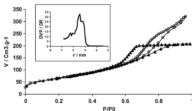
Fig. 3 Nitrogen adsorption-desorption isotherms of samples **2** ( $\blacktriangle$ ) and TiO<sub>2</sub> ( $\circ$ ) and pore size distribution vs. radius (inset).
