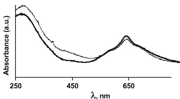
**Fig. 4** DR UV–Vis spectra of initial FePcS–TiO<sub>2</sub> (bold line) and after 3 oxidations (light line).
