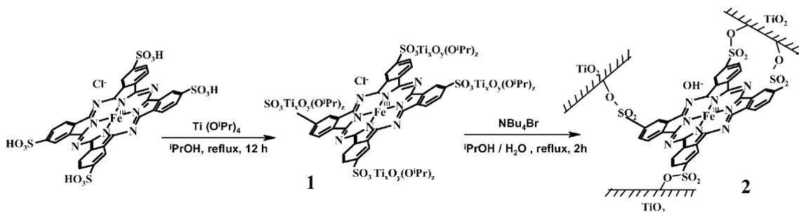
Fig. 1 Preparation of FePcS-TiO<sub>2</sub> (2).
