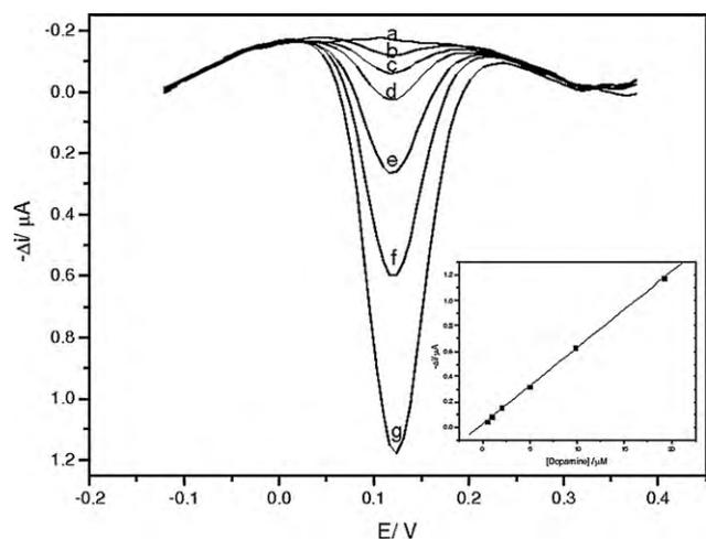
**Fig. 5.** Square wave voltammograms obtained using the biomimetic sensor for (a) blank in phosphate buffer solution (pH 8.0), and dopamine solutions at the following concentrations: (b)  $4.99 \times 10^{-7}$  M; (c)  $9.98 \times 10^{-7}$  M; (d)  $1.99 \times 10^{-6}$  M; (e)  $4.95 \times 10^{-6}$  M; (f)  $9.80 \times 10^{-6}$  M and (g)  $1.92 \times 10^{-5}$  M in 0.1 M phosphate buffer solution (pH 8.0).
