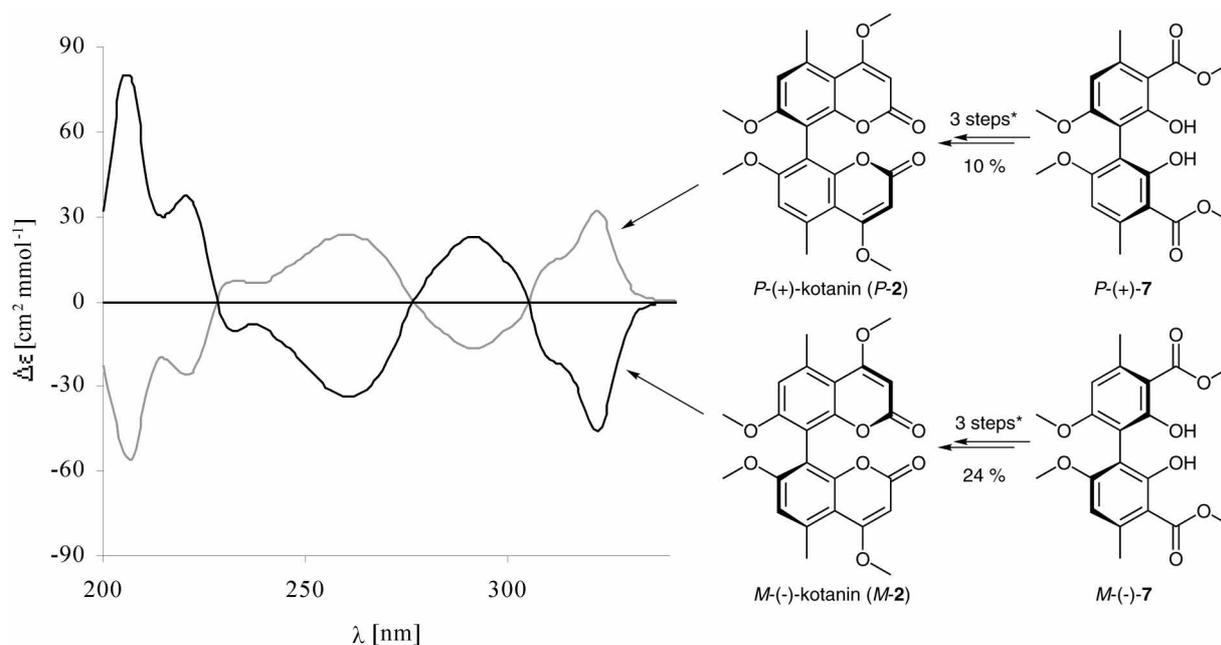
**Scheme 5** Syntheses of *P*- and *M*-kotanin (**2**) and CD spectra (acetonitrile) (\*For reaction conditions, see Scheme 4)
