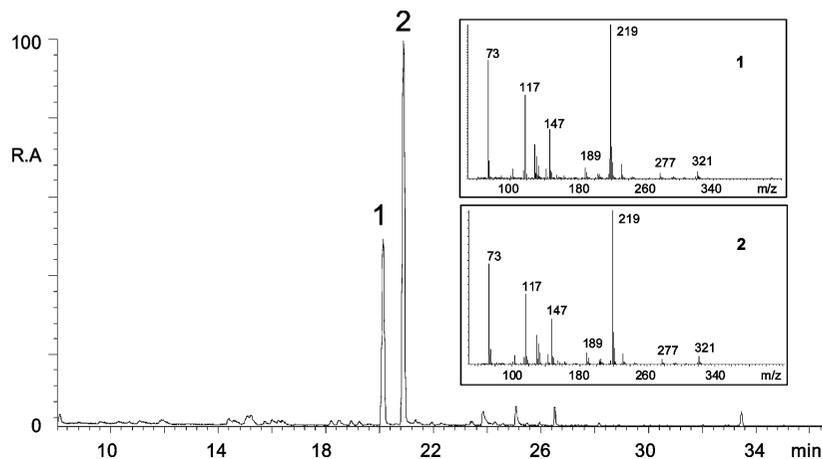
**Figure 1.** GC/MS total ion chromatograms obtained for the reaction mixtures of isoprene with  $\text{H}_2\text{O}_2$  and sulfuric acid derivatized by BSTFA and spectra for products (insets) **1** (2-methylthreitol) and **2** (2-methylerythritol).
