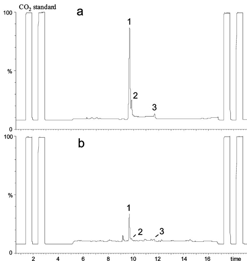
**Figure 3.** GC/C/IRMS chromatogram of 2-methyltetrol–MBA derivatives: (a) standard derivative and (b) extract of the fine size fraction of a 24 h Hi-Vol aerosol sample collected at Dinghu, China, on August 2, 2006. Compounds **1** and **2** are 2-methylerythritol–MBA derivatives, and compound **3** is the 2-methylthreitol–MBA derivative.
