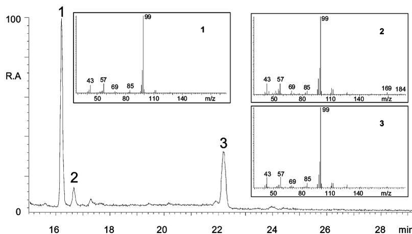
**Figure 2.** GC/MS total ion chromatogram obtained for 2-methyltetrols derivatized by MBA and mass spectra for the products (insets). Compounds **1** and **2** correspond to 2-methylerythritol–MBA derivatives, and compound **3** corresponds to a 2-methylthreitol–MBA derivative.
