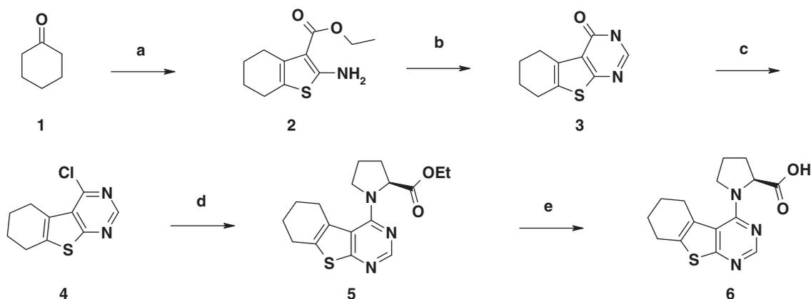
**Scheme 1** Synthetic route for 1-(5,6,7,8-tetrahydro-benzo[4,5]thieno [2,3-d]pyrimidin-4-yl)-pyrrolidine-2-carboxylic acid (**6**). Reagents and solvents: **a** ethyl cyanoacetate, sulphur, morpholine, EtOH, Reflux;
