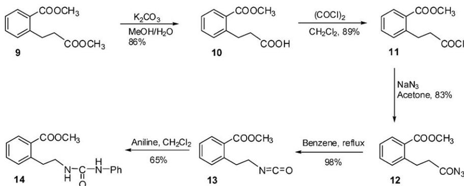
Fig. 3. Synthesis of urea derivative **14** starting from the diester **9**.
