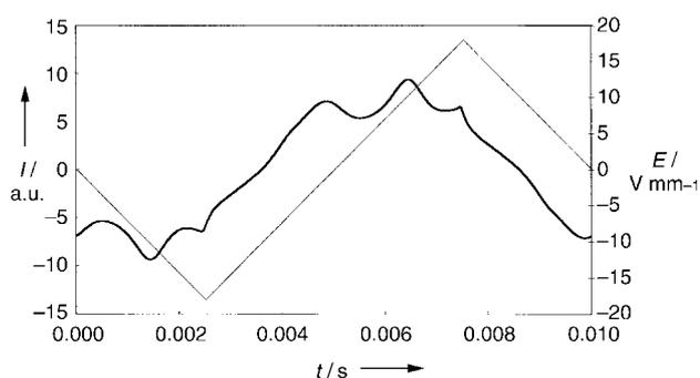
**Figure 3.** Polarization switching current of complex **1.3** under a triangular-wave electric field: 100 Hz, 36 Vpp μm<sup>-1</sup> (5 μm-Linkam cell).
