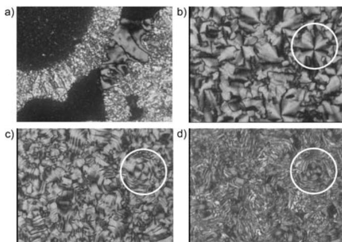
**Figure 1.** Textures of the mesophase SmCP: a) Complex **2.3** at 144 °C, uncoated cell; b) complex **1.3** at 100 °C,  $V=0$ , coated cell; c) complex **1.3** at 100 °C,  $V=70$  (d.c.), coated cell; d) complex **1.3** at 100 °C,  $V=100$  (d.c.), coated cell. The orientation of the extinction brushes is seen clearly in the circles indicated.
