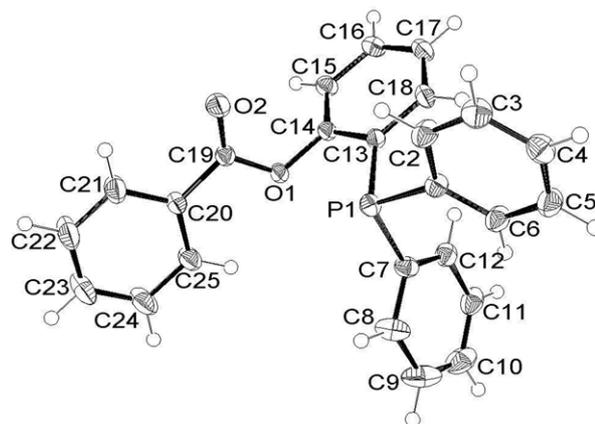
**Figure 1** Molecular structure of compound **4a** (ORTEP-Plot, 50% probability level). Selected bond lengths (Å) and angles (°): P1–C1 1.8358(8), P1–C13 1.8339(8), P1–C7 1.8343(9), O2–C19 1.2060(10), O1–C19 1.3618(9), C19–O1–C14 116.01(6), O2–C19–O1 122.88(7), C13–P1–C7 101.65(4), C13–P1–C1 101.11(3).
