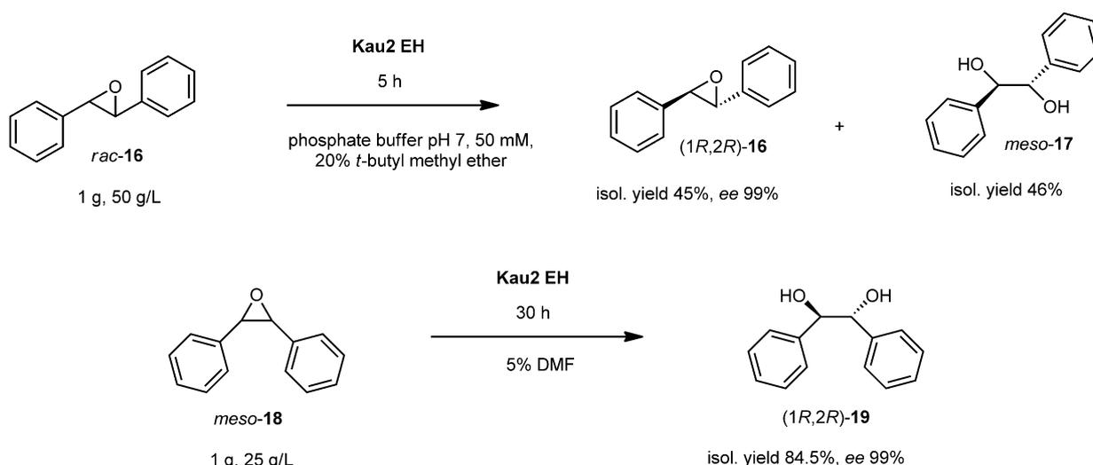
**Scheme 5.** Kinetic resolution of *trans*-stilbene oxide (**16**) and desymmetrization of *cis*-stilbene oxide (**18**).
